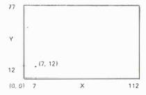
Example: PLOT (7, 12, 3) plots color 3 at point (7, 12), as shown in the diagram.
